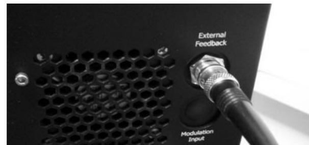
Figure 9: Electrical interface at the back of the SuperK EXTREME
