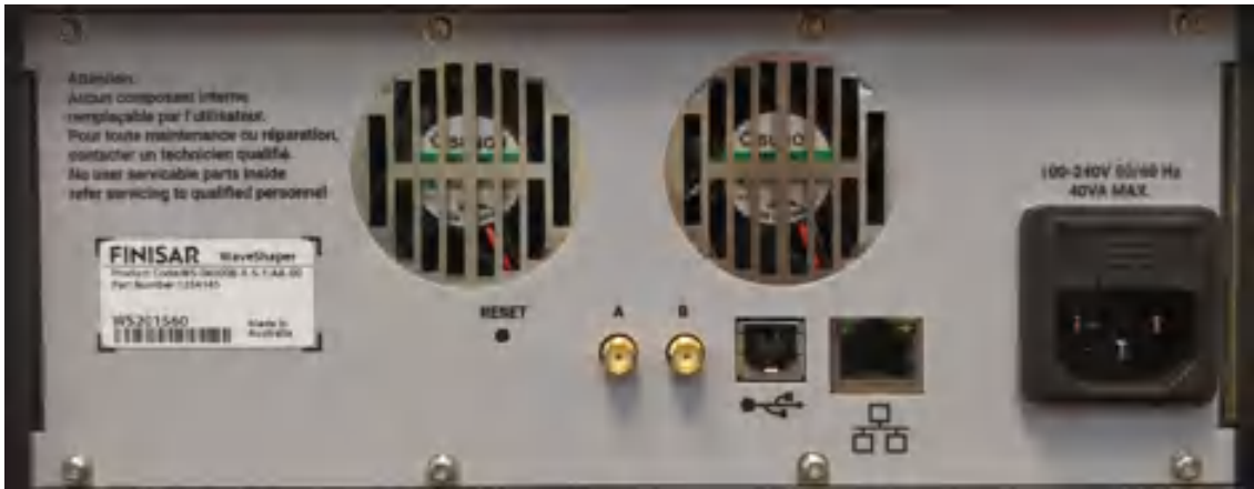
Rear view of the Series B benchtop showing the power supply, fan, USB, Ethernet, reset button and serial number. Note the SMA connectors are not used.
