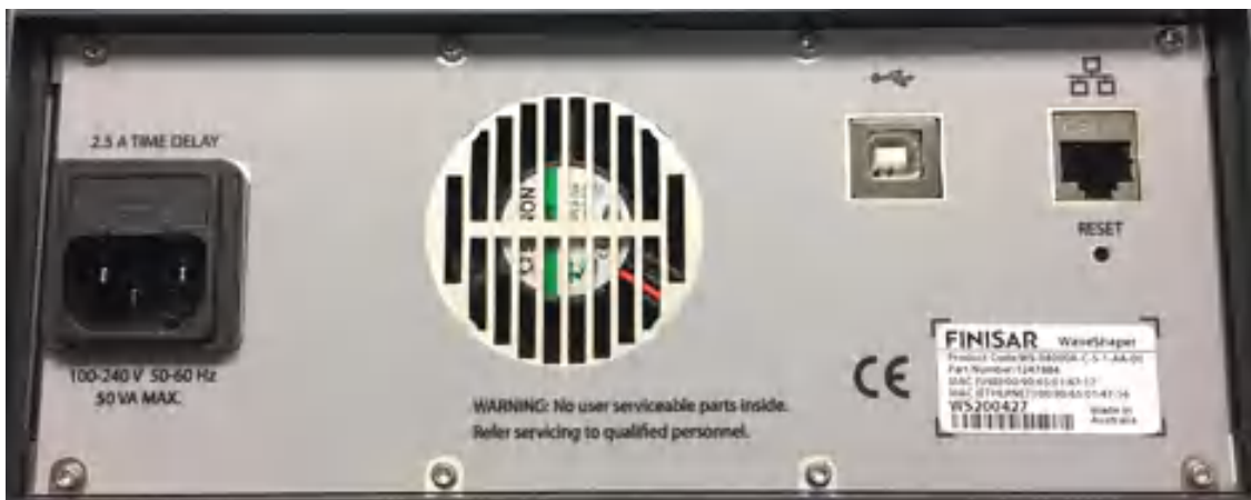
Rear view of the Series A benchtop showing the power supply, fan, USB, Ethernet, reset button and serial number.
