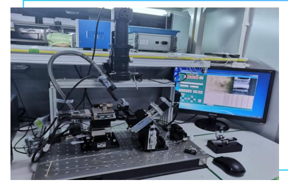
Automatic Collimator Alignment
