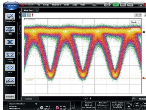
DPSK Output optical signal
