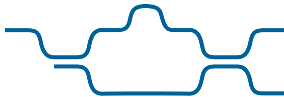
Figure 2: Variable Delay Line Interferometer
