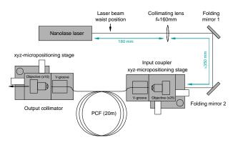
Fig. 3: Schematic of experimental setup
