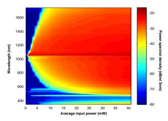
Fig. 9.: Power spectral density at the end of 20m of PCF as a function of average pump power in the fiber (Pulse width 600 ps, repetition rate  $\approx$ 7 kHz) [6]
