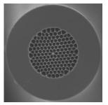
Fig.10 (a): Solid core PCF. This example shows a fiber designed to provide high non-linearity by strongly confining the light in the small central core. Such fibers can be used to create supercontinuum radiation from the femtosecond output of a Ti:Sapphire laser at 800 nm wavelength.
