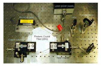
Fig. 4: Experimental setup, including Teem Photonics Nanolase<sup>™</sup> microchip-laser, input and output coupling optics.
