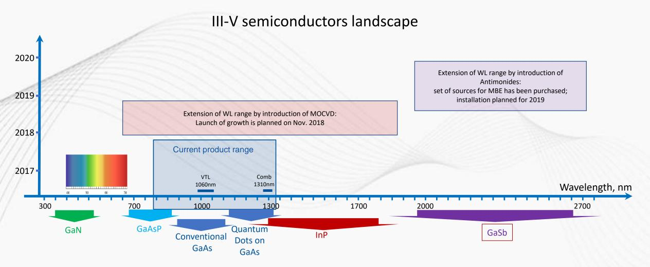
Extension of materials to InP- & GaSb-based systems will enable new design of laser products for novel applications
